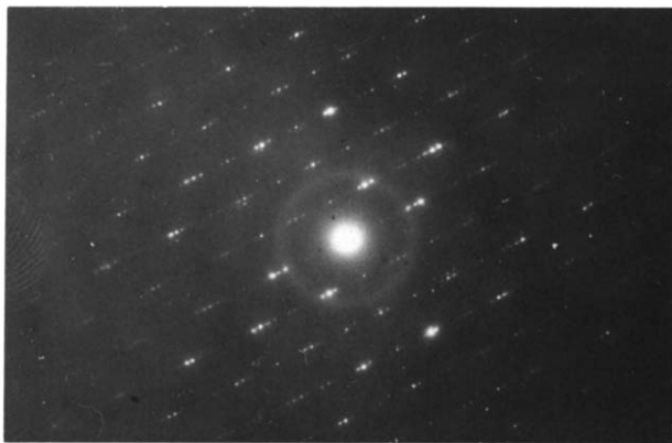
Fig.3. SADP for intergrain space of crystallized material.
